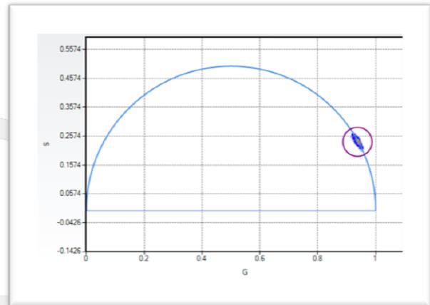
Cell expressed with Cerulean. Excitation wavelength was 488 nm from a pulsed laser diode. The phasor plot collects the pixels of the image; a decay time of 4 ns is measured.
