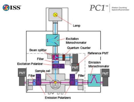
Figure 2. Schematic drawing of PC1, the photon-counting spectrofluorimeter from ISS.
