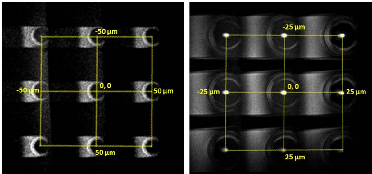
**Figure 4:** Overlay of the images of the Nanowizard tip at 9 different positions by Q2, using Olympus 20X / 0.75 NA (left) and 60X / 1.2 NA water (right) objective lenses.
