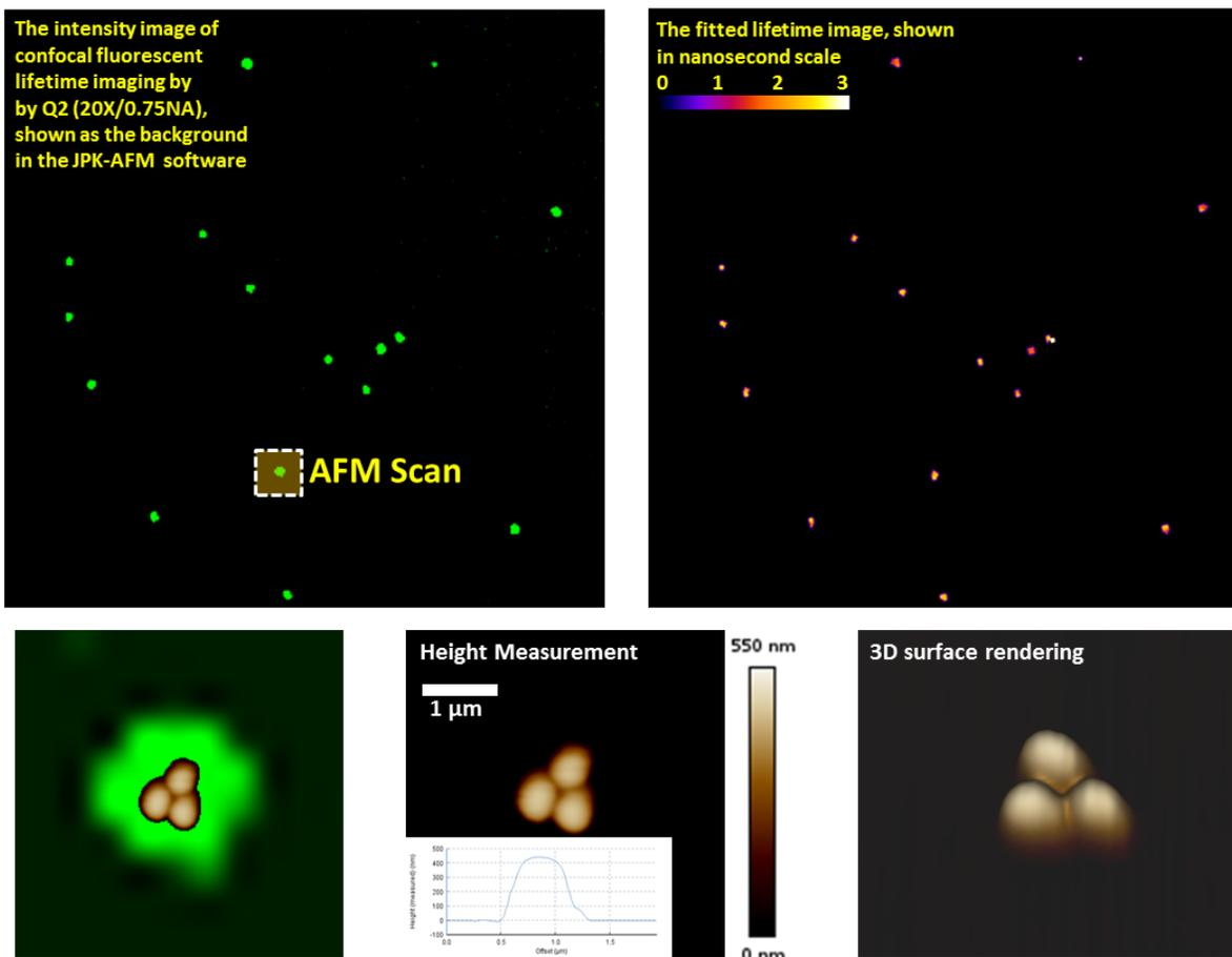
**Figure 5:** Correlative Confocal FLIM-AFM measurements of fluorescent beads.
