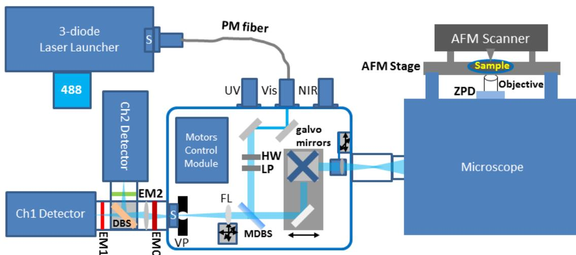
**Figure 3:** The system schematic combining ISS Q2 and JPK Nanowizard. HW: halfwave plate; LP: linear polarizer; MDBS: main dichroic beam splitter; VP: variable pinhole (motorized and continuously tunable from 20 to 1000  $\mu\text{m}$ ); S: Shutter; EM0, EM1, EM2: emission filters; DBS: dichroic beam splitter; ZPD: Z-Piezo device.
