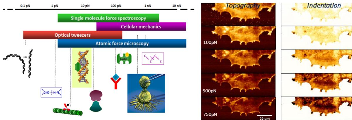
**Figure 2:** The diagram (Left) depicts the forces for biological process from molecular interactions to cell mechanics. JPK's AFMs and Optical Tweezers can address the range from a few pN to hundreds of nN. Shown on the right are data from living COS-7 cells from a force cube obtained using QI in a petri dish heater. The topographic and corresponding indentation images reveal useful information topography and mechanical properties of the cell.
